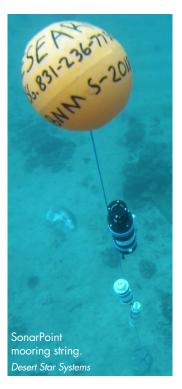
recorders. Recorder depth locations will test the signal detection and localization capabilities for cetaceans vocalizing at varying depth distances from the recorders. Depth and spacing results will be used to configure recorders for the second deployment. The project team will validate array recordings by using a variety of standard visual and passive acoustic methods to detect, approach and record a variety of species, and determine their positions.
